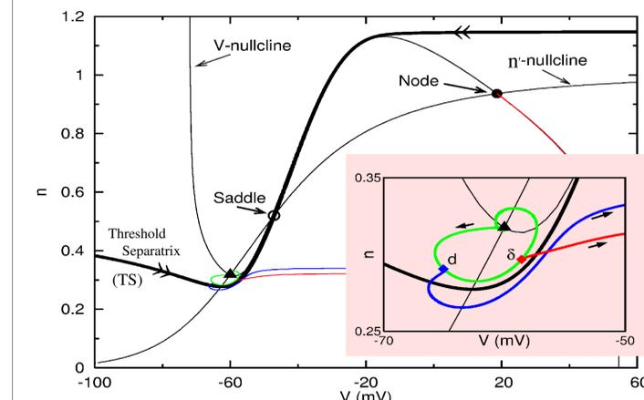
A 2D reduced HH model with  $m = m_\infty(V)$  and  $h = h_{rest}$  (constant) gives a phase-plane view of the two main mechanisms, PIF and PIR.
